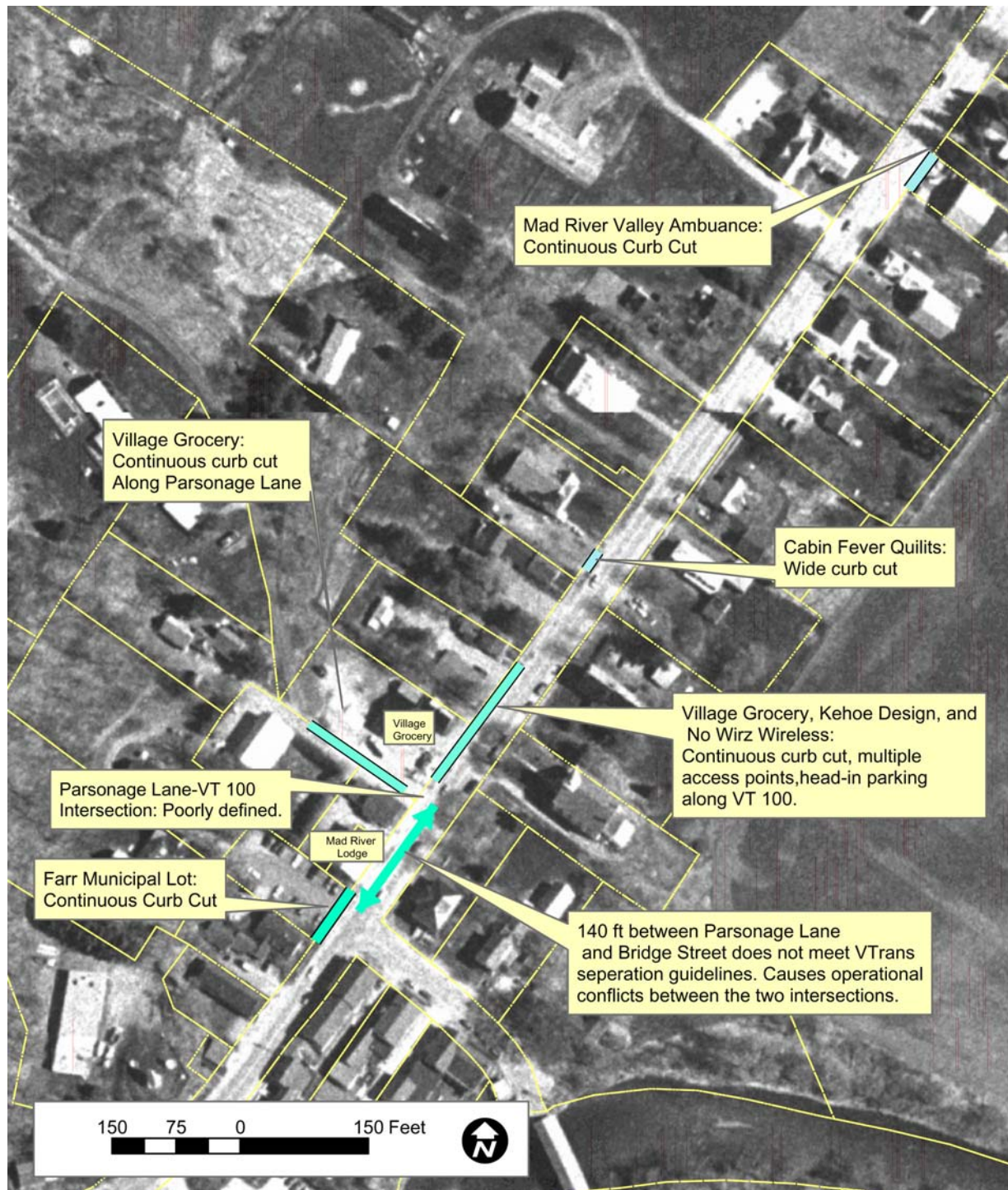
Figure 13: Access Management Issues
